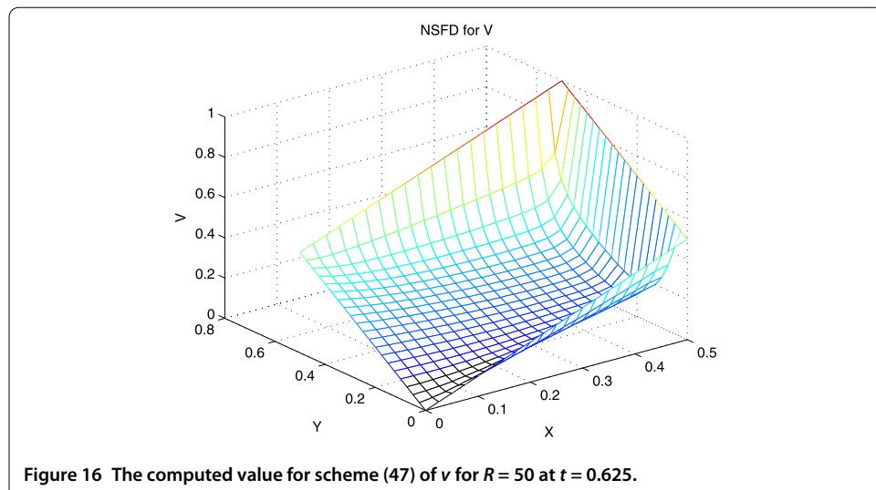
**Figure 16** The computed value for scheme (47) of  $v$  for  $R = 50$  at  $t = 0.625$ .
