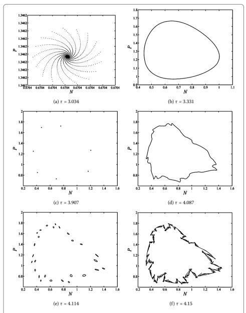
**Figure 2** Phase diagrams corresponding to the bifurcation diagram in Fig. 1(a), demonstrating the dynamic transition on the route to chaos induced by the Hopf bifurcation
