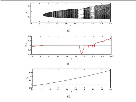
**Figure 1** Diagrams of (a) Hopf bifurcation, (b) maximum Lyapunov exponent (MLE), and (c)  $\lambda_m$ , demonstrating the change of dynamical properties of the discrete system corresponding to variation of parameter  $\tau$ . r = 0.8, K = 1.8,  $\beta = 0.6$ ,  $\varepsilon = 1$ ,  $\beta = 0.4$ , w = 0.4,  $\eta = 0.25$ ,  $C_1 = 0.1$ ,  $C_2 = 0.01$ ,  $D_1 = 0.01$ ,  $D_2 = 0.1$ ,  $D_3 = 0.01$ ,  $D_4 = 0.01$ ,  $D_5 = 0.01$ ,  $D_6 = 0.01$ ,  $D_7 = 0.01$ ,  $D_8 = 0.01$ ,  $D_9 =$
