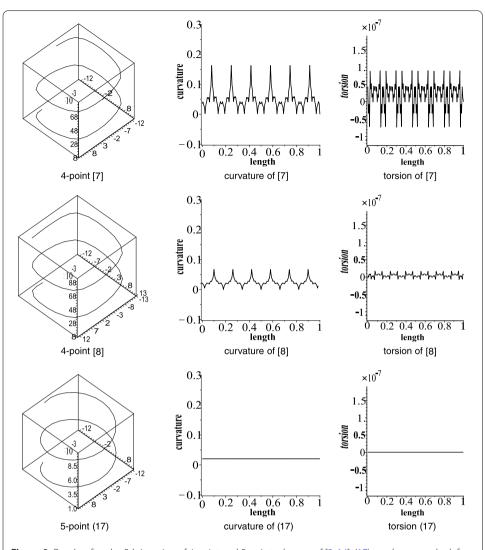
Figure 8 Results after the 5th iteration of 4-point and 5-point schemes of [8, 14], (17) are shown on the left when the initial control points are sampled from Helix. The corresponding curvature and torsion are shown in the center and right columns, respectively
