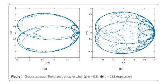
By taking a = 1 and b = 0.83, system (8) exhibits a chaotic behavior, which is shown in Fig. 1(a). When b is further increased to 0.88, a more complex chaotic attractor is plotted in Fig. 1(b).
