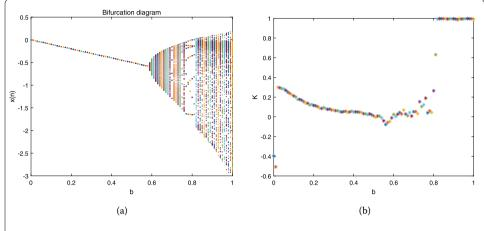
**Figure 2** Bifurcation diagram and K median value. The bifurcation diagram (**a**) and K median value (**b**) of system (10) with a = 1, v = 0.9 versus parameter b
